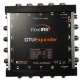
The GTU Expander can increase the output from a Quatro GTU from 8 to 48 outputs (when using 3 x 16 way expanders in cascade). Its unique design allows it to be connected directly to the Quatro GTU without using additional cables.
